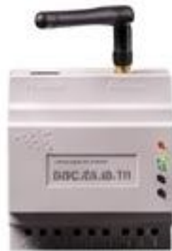
Gateway Signal Receiver The data acquisition and communication hub.
